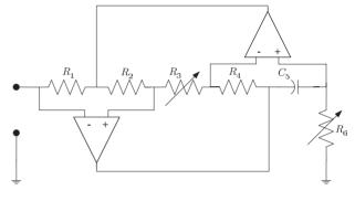
Figure 7. Schematics of the grounded inductor.
