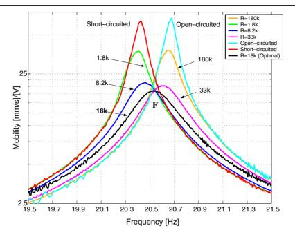
Figure 11. Experimental mechanical mobility around the first mode for the R network with different line resistances.
