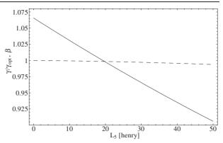
**Figure 6.** Tuning and coupling parameters  $\beta$  (solid line) and  $\gamma$  (dashed line) as functions of the terminal inductance when the line inductance is fixed to 130.5 H.
