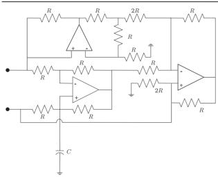
Figure 5. Schematics of the floating inductors.
