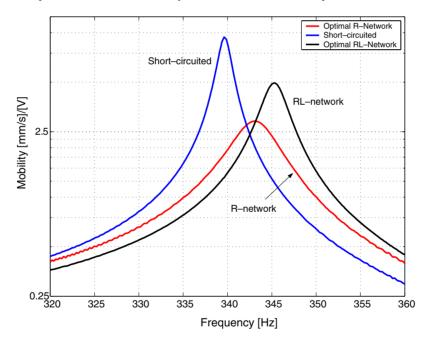
Figure 10. Experimental mechanical mobility around the third mode for optimal R and RL networks.
