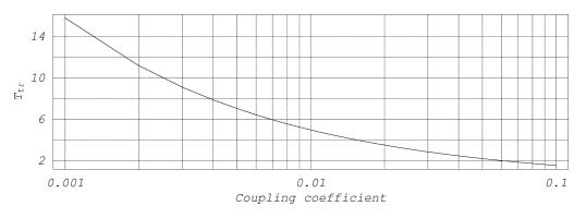
**Figure 4.** Elapsed time to transfer energy  $T_{tr}$  as a function of the coupling coeff cient k.
