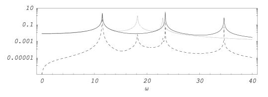
Figure 12. Plots of the mechanical (black), electrical (gray) and electro-mechanical (dashed) frequency-response functions. The impedance is set to the optimal value for mode 1.
