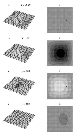
Figure 16. Mechanical (left column) and electrical (right column) vibrations induced in the piezo-electromechanical plate by an impulse concentrated at the point  $P_2$ . Its localization is specifie by the black dot. Electric potential is represented as a black–white scale: gray means ground, non-dimensional time is indicated.
