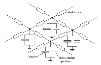
Figure 2. Electrical connection scheme.
