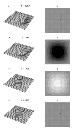
Figure 14. Mechanical (left column) and electrical (right column) vibrations induced in the piezo-electromechanical plate by an impulse concentrated at the point  $P_1$ . Its localization is specifie by the black dot. Electric potential is represented as a black–white scale: gray means ground, non-dimensional time is indicated.
