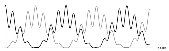
Figure 5. Electric (gray) and mechanical (black) energies vs. time.
