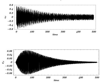
Figure 17. Time evolution of displacement and electric state at a representitive point of the piezoelectromechanical plate, with impulse concentrated at  $P_2$ .
