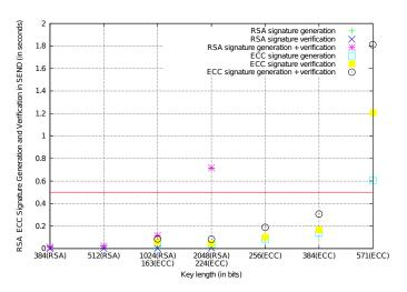
Figure 9: Comparison between CGA/RSA and CGA/ECC signature generation and verification on a Nokia N800
