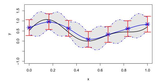
Figure 15: Kriging with homogeneously noisy observations
