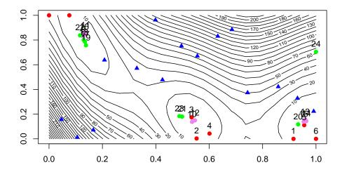
Figure 30: Parallelized EGO for the Branin function. 3 iterations of Constant Liar with 8 parallel searches.
