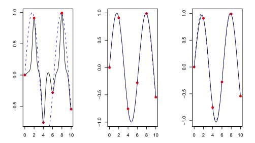
Figure 19: Comparison of three estimation methods for Kriging approximation of the sine function, with 6 design points: MLE (left), PMLE with SCAD penalty (middle), MLE constrained by  $\theta \geq 10/5$  (right). The bullets represent the design points, the solid line the Kriging mean and the dotted line the sine function.
