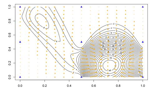
Figure 22: Gradient field of the EI associated to a Kriging metamodel of the Branin function
