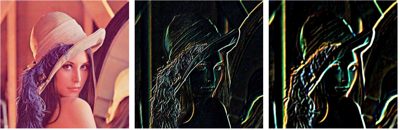
Figure 1: Original image, derivatives with Hann kernel \tilde{s}_H(t) = 2s_H(2t) and s_{H,1/4}(t) = \frac{1}{2}s_H(\frac{1}{4}t) ( \varphi = \frac{2\pi}{3} ).
