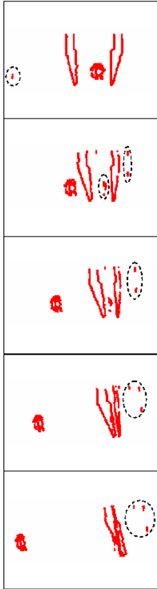
Figure 6: Novel views with the angle \alpha varying from 0^\circ to 80^\circ : the gripper is over the gear. The surrounded elements correspond to errors of matching.
