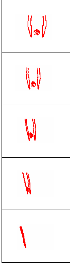
Figure 8: Novel views with the angle \alpha varying from 0^\circ to 80^\circ : the gear is within the gripper.
