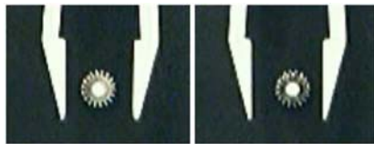
Figure 5: Input left and right views respectively: the gripper is over the gear.
