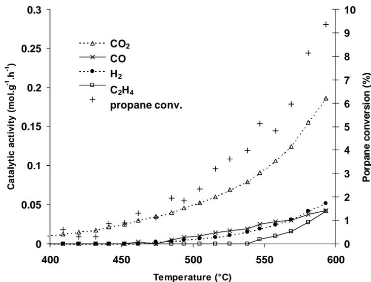
Figure 3: Catalytic activity of GDC (15 mg; 10%wt in alumina) as a function of temperature, with an O<sub>2</sub> / C<sub>3</sub>H<sub>8</sub> ratio equal to 6/4.
