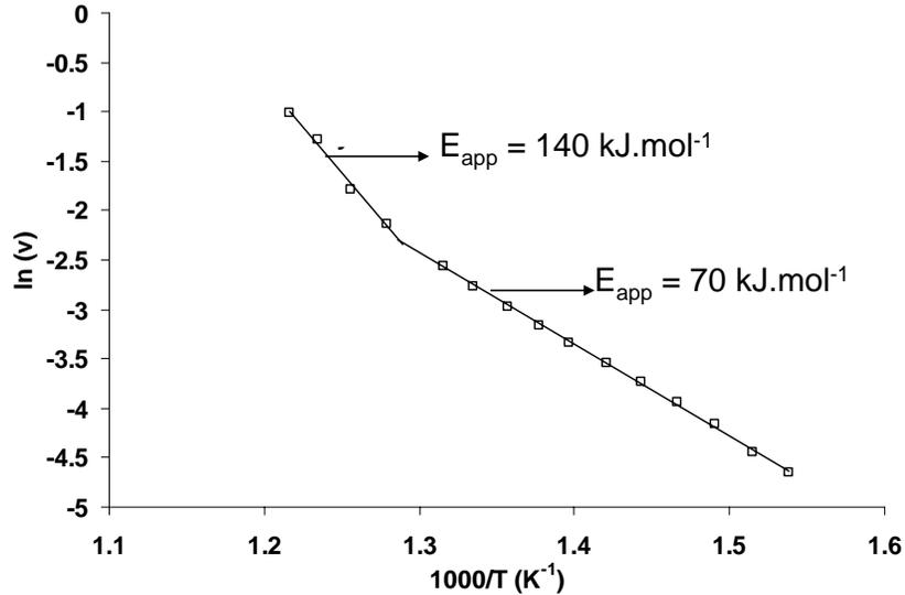
Figure 8 : Arrhenius plot of carbon dioxide production calculated from the experiment (O<sub>2</sub> / C<sub>3</sub>H<sub>8</sub> equal to 6/4)
