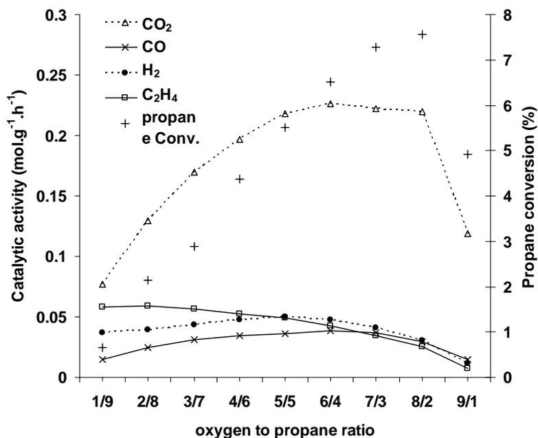
Figure 2: Catalytic activity of GDC (15 mg; 10%wt in alumina) at 590°C, as a function of the O<sub>2</sub>/C<sub>3</sub>H<sub>8</sub> ratio.
