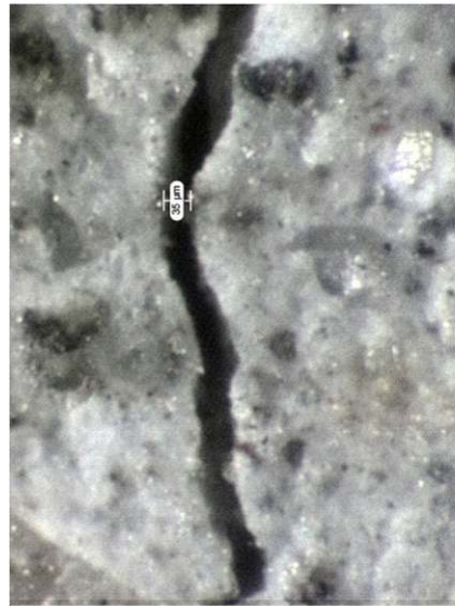
b) \text{COD}_{\text{max}} = 105 \text{ } \mu\text{m} , w_1 \approx 35 \text{ } \mu\text{m}
