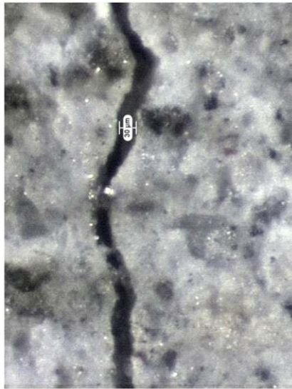
a) \text{COD}_{\text{max}} = 80 \text{ } \mu\text{m} , w_1 \approx 30 \text{ } \mu\text{m}
