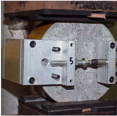
Fig. 2. COD measurement during loading.
