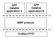
Figure 3. The Network Protocol Stack
