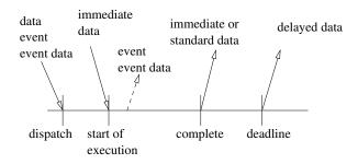
Figure 2. communication through ports in AADL.
