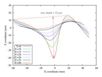
Fig. 11 Profiles along X-axis for different Y values after springback. The simulation is performed with shell elements
