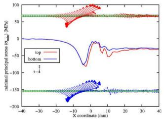
Fig. 12 Distribution of the minimum principal stress (in MPa) in the bottom and top layers of the blank, at Y = 7 mm, for solid elements. The top surface is the one in contact with the blankholder and the bottom surface with the die. The orientation of the corresponding principal direction is also given
