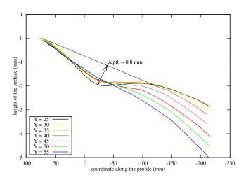
Fig. 8 Profiles after springback for the second refinement at different Y coordinates
