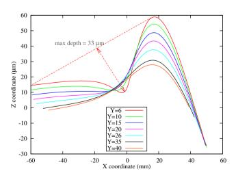
Fig. 10 Profiles along X-axis for different Y values after springback. The simulation is performed with solid elements
