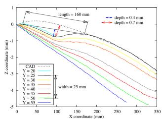
Fig. 4 Profiles of the Atos measurement on the upper corner surface
