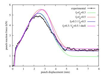
**Fig. 9** Comparison of the numerical and experimental punch reaction force with different configurations of numerical friction coefficients for DP500 with a flanged length of 2.5 mm
