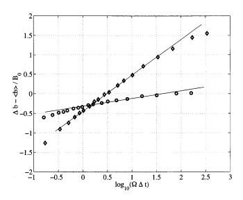
FIG. 12. Evolution of the peak to peak value of the magnitude of the induced magnetic field  $[\delta b(\Delta t) = \max(b) - \min(b)]$  as the interval  $\Delta t$  over which it is calculated increases. Two experiments are shown ( $\bigcirc$ ): disks rotating at 8 Hz ( $R_m = 20$ ) and ( $\diamondsuit$ ): disks' rotating at 17 Hz ( $R_m = 43$ ). The straight line corresponds to a logarithmic evolution  $\delta b(\Delta t) \propto B_0 \log \Omega \Delta t$ .
