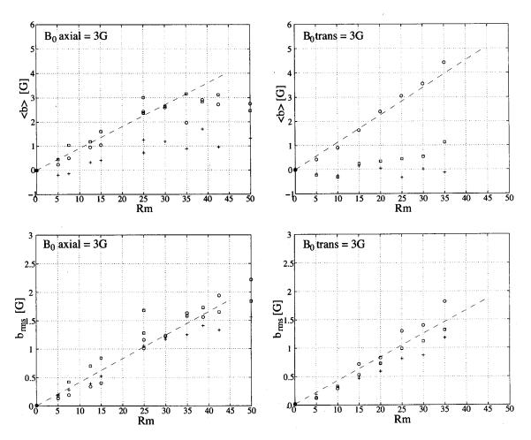
FIG. 8. Mean and standard deviations of the induced field as a function of the magnetic Reynolds number of the flow. (Left-hand side) Axial  $B_0=3$  G, and (right-hand side) transverse  $B_0=3$  G. (O) Axial component  $b_x$  of the induced field, ( $\Box$ ) transverse component  $b_y$ , (+) vertical component  $b_z$ . The measurement probe is located near the midplane, 10 cm away from the axis of rotation.
