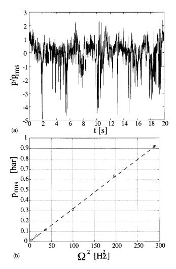
FIG. 5. (a) Time variation of the pressure measured at the flow wall ( $\Omega$ =17 Hz); (b) evolution with the disks' rotation rate of the rms amplitude of the pressure fluctuations. The dashed line corresponds to the quadratic law  $p_{\rm rms}/\Omega^2$ =3.2×10<sup>-3</sup> [bar/Hz<sup>2</sup>].
