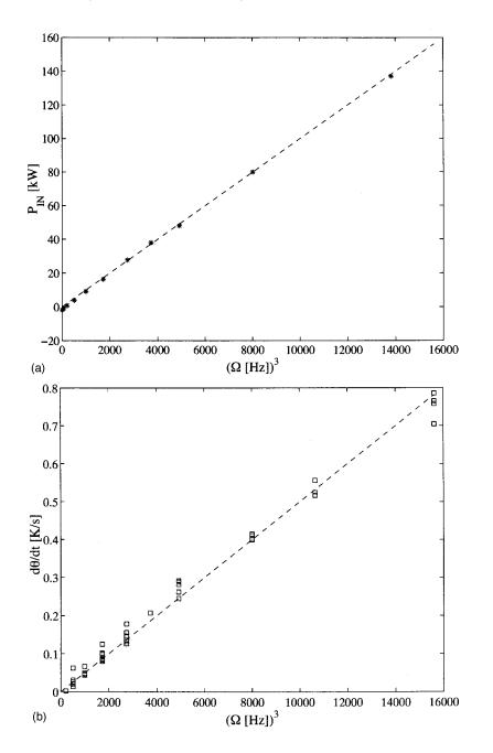
FIG. 6. Variation of the power input in the flow measured (a) from mechanical power delivered the motors (a cubic law best fit yields  $P/\Omega^3 = 10^{-2} [kW/Hz^3]$ ) and (b) from the increase of the temperature inside the flow vessel during one experiment (here, a cubic law fit yields  $d\theta/dt/\Omega^3 = 5 \times 10^{-5} [K/s/Hz^3]$ ).
