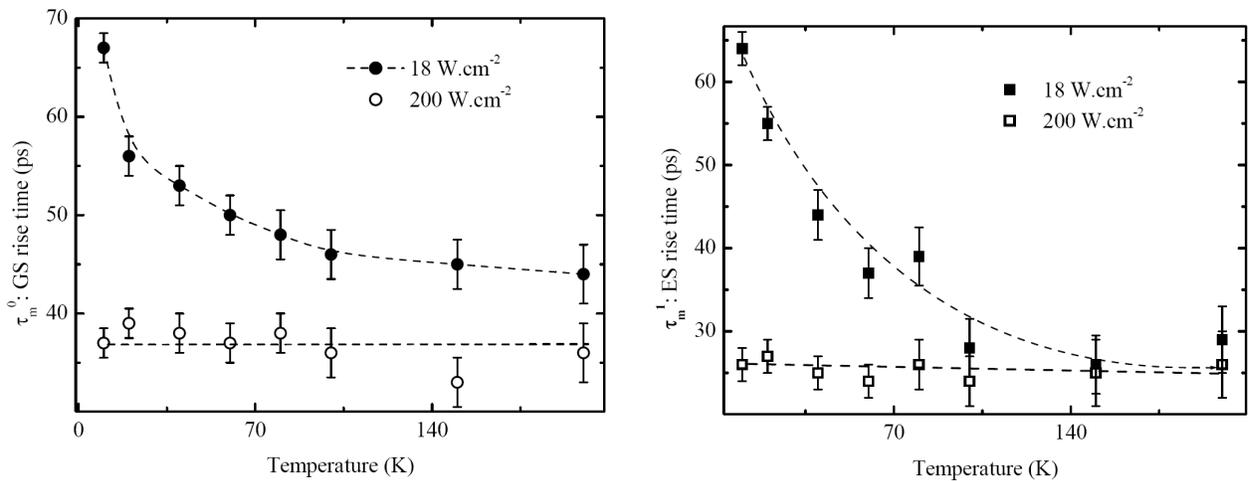
Figure 4. GS (left) and ES (right) rise times as a function of temperature for weak (18 W.cm<sup>-2</sup>) and strong (200 W.cm<sup>-2</sup>) excitation densities.
