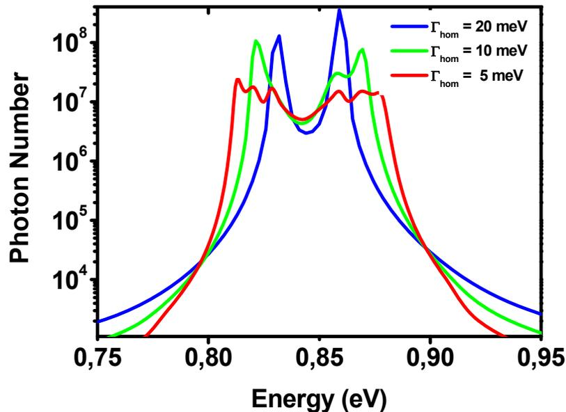
Figure 5. Calculated lasing spectra showing two-state laser emission at fixed current injection for different values of the homogeneous broadening width
