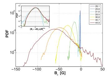
FIG. 13. (Color online) PDFs of local fluctuations of  $B_{\theta}$ . Measurement at point P1, VKS2h. Magnetic Reynolds numbers are given in the legend and profiles below onset cannot be distinguished. Inset: PDFs for centered and normalized variables.
