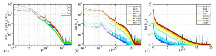
FIG. 16. (Color online) Time spectra of magnetic field fluctuations at point P1. (a) Three components,  $R_m \sim 40$ ; [(b) and (c)] log-log plot and semilog plots of  $B_x$  spectra for increasing  $R_m$  values.
