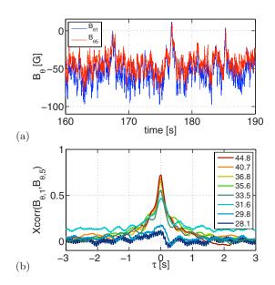
FIG. 5. (Color online) Magnetic field measured at points P1 and P5 in VKS2h: (a) Time traces of the azimuthal magnetic field components. (b) Cross correlation function of the two signals for increasing magnetic Reynolds numbers in the range of 28–45.
