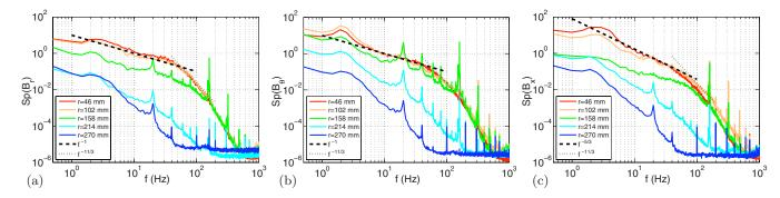
FIG. 14. (Color online) Time spectra of magnetic field fluctuations measured with the probe array at point P3 (location of the innermost sensor) in VKS2i. Different curves on each plot correspond to different sensor depth, labeled in the legend by their distance r to the rotation axis. The rotation frequency of the impellers is 20 Hz: (a) Axial component, (b) azimuthal component, and (c) radial component.
