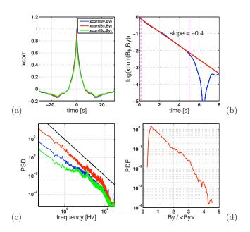
FIG. 24. (Color online) Bursting regimes, VKS2h;  $F_1$ =22 Hz,  $F_2$ =15 Hz,  $\Theta$ =0.19 [cf. Fig. 23]. (a) Time correlations of the magnetic field components. (b) log-linear plot of the autocorrelation of the largest field component  $\langle B_y(t)B_y(t+\tau)\rangle_t$ . (c) Corresponding time-power spectra—the black solid lines shows an  $f^{-2}$  scaling. (d) PDF for  $B_y(t)$ .
