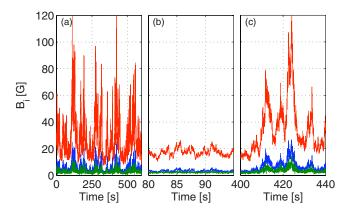
FIG. 23. (Color online) (a) Bursting regimes, VKS2h;  $F_1$ =22 Hz,  $F_2$ =15 Hz,  $\Theta$ =0.19; three components of the magnetic field measured at point P1 [blue: axial component; red: minus azimuthal component; and green: radial component; see legend of Fig. 2(a)]. (b) and (c) are zoomed on, respectively, quiet periods and active bursts.
