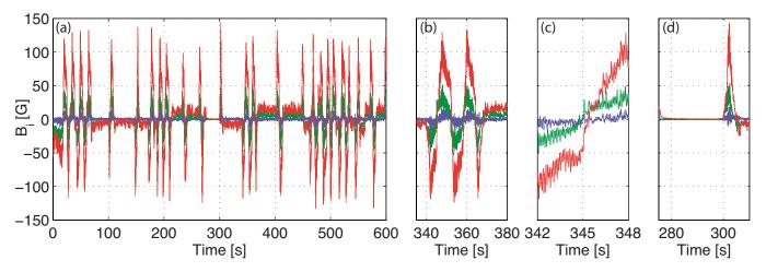
FIG. 25. (Color online) Bursting regimes, VKS2h;  $F_1$ =21 Hz,  $F_2$ =15 Hz, and  $\Theta$ =0.167. (a) Three components of the magnetic field measured at point P1 [blue: axial component; red: azimuthal component; and green: radial component; see legend of Fig. 2(a)]. (b) and (c) are further zoomed on the oscillations (note the change in polarity of the low state mode before and after the oscillations). (d) Zoom including the ending extinction around t=300 s.
