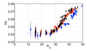
FIG. 10. (Color online) Evolution with  $R_m$  of the power number defined in Eq. (7) and measured from the drives of the motors. The blue circles (and dashed line as an eye guide) are from nondynamo runs (VKS2f) with stainless steel impellers. The red stars (VKS2g) and black squares (VKS2h) come from two dynamo runs, with same geometry but with soft-iron impellers and also without any magnetic probes in the flow bulk.
