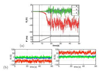
FIG. 2. (Color online) Three components of the magnetic field generated by dynamo action at  $F_1$ = $F_2$  measured at point P1 in the experiment VKS2g. (a) Growth of the magnetic field as the impellers' rotation rate F is increased from 10 to 22 Hz. (b) Two independent realizations at same frequency above threshold showing opposite field polarities.
