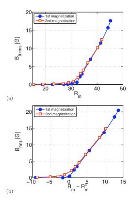
FIG. 11. (Color online) Evolution with  $R_m$  of rms values of the magnetic field at saturation. Measurements at point P1 in VKS2h. (a) Azimuthal component  $B_{\partial \text{rms}}$ . (b) Magnetic field amplitude  $B_{\text{rms}}$ . The closed blue circles corresponds to a first run with almost demagnetized impellers (see text) and the open red squares to the subsequent runs.
