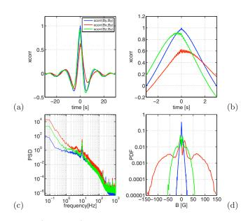
FIG. 26. (Color online) Bursting regimes, VKS2h;  $F_1$ =21 Hz,  $F_2$ =15 Hz,  $\Theta$ =0.167 [cf. Fig. 25]. (a) Time correlations of the magnetic field components. (b) Zoom around zero time lags. (c) Corresponding time-power spectra. (d) PDFs of the three magnetic field components. Color code for (c) and (d) as in Fig. 25.
