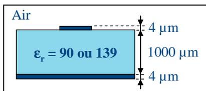
Figure 2. Configuration microruban.
