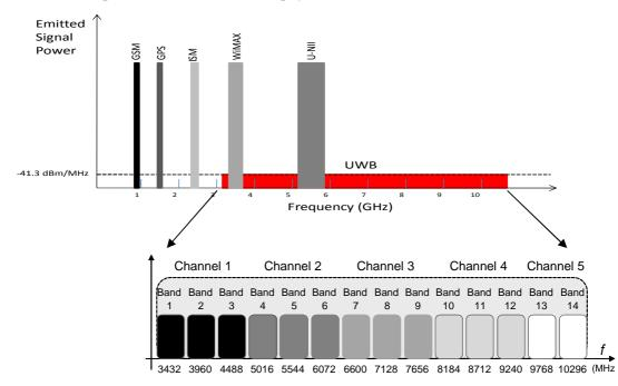
Fig. 1. UWB spectrum and sub-band distribution for WiMedia solution.
