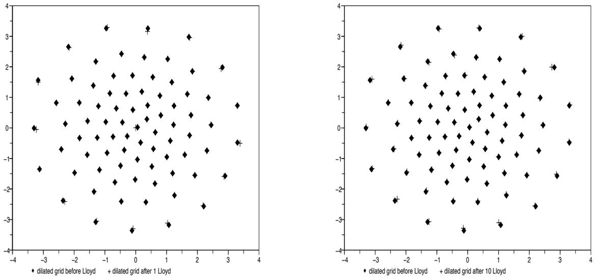
Figure 2: The  $L^2$ -dilated grid before and after 1 and 10 Lloyd's iterations; the grid size equals 80.
