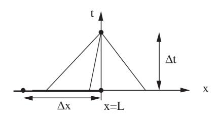
Figure 4 Nonreflecting output at x = L.
