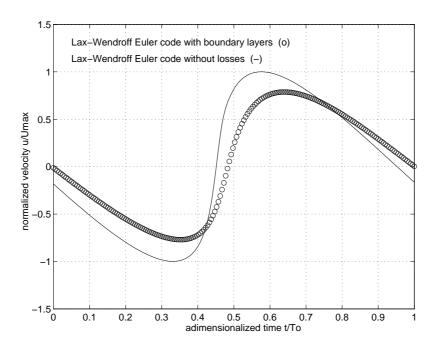
**Figure 10** Comparison of flow field at s = 0.8 with and without loses
