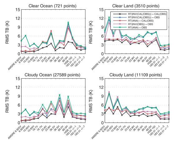
FIG. 8. RMS differences between RTM simulations and calibrated (or noncalibrated) real observations. The RMS errors are for RT(ana) - obs (green), RT[INV(obs)] - CAL(obs) (purple), RT(ana) - CAL(obs) (red), RT[INV(obs)] - obs (blue), and  $RT\{INV[CAL(obs)]\} - CAL(obs)$  (black). See the text and Table 2 for explanations.
