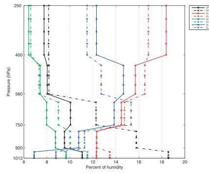
FIG. 5. RMS relative humidity departure of the ECMWF analysis and the retrieval from raw (dotted) and calibrated (solid) *Aqua* observations for cloud free/land (black), cloudy/land (green), cloud free/ocean (red), and cloudy/ocean (blue) configurations.
