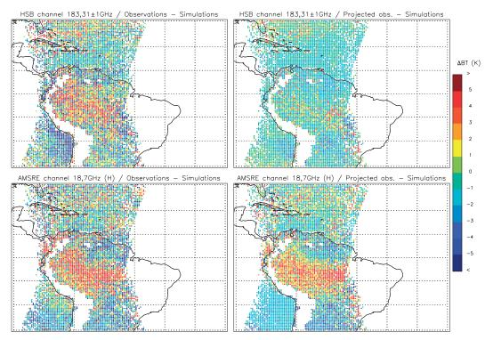
FIG. 3. RMS error maps computed over two months for differences between RTTOV simulations and (left) real Aqua observations and (right) calibrated Aqua observations for (top) an HSB channel at 183.31  $\pm$  1 GHz and (bottom) an AMSR-E channel at 18.7 GHz, vertically polarized.
