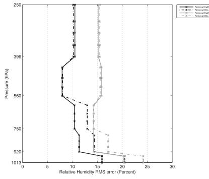
FIG. 6. RMS differences in relative humidity between a collection of radiosonde measurements and coincident retrievals from raw (dot–dashed) and calibrated (solid) *Aqua* observations. These statistics are performed over land for clear (gray) and cloudy (black) scenes over two months over the tropics.
