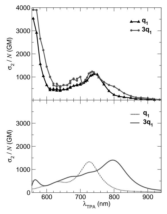
Figure 18: TPA cross section of chromophores  $3q_1$  and  $q_1$  normalized for the number of branches (N). Top panel: experimental data in toluene; Bottom panel: calculated cross section in vacuum, but corrected for local field and refractive index. Adapted from.<sup>[126]</sup>
