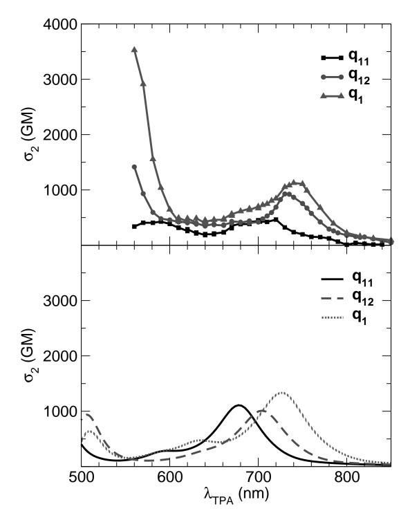
Figure 13: TPA cross section of chromophores  $q_1$ ,  $q_{11}$  and  $q_{12}$ . Top panel: experimental data in toluene; Bottom panel: calculated cross section in vacuum, but corrected for local field and refractive index. Adapted from.<sup>[126]</sup>
