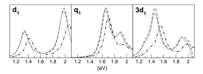
Figure 8: TPA cross sections (arbitrary units) of dipolar  $(d_1)$ , quadrupolar  $(q_1)$  and 3-branched octupolar  $(3d_1)$  chromophores obtained with different models for the second-order hyperpolarizability  $(\gamma^{sol})$ : vac-vac (dashed-dotted line), vac-tol (dashed line) and tol-tol (continuous line) (see main text).
