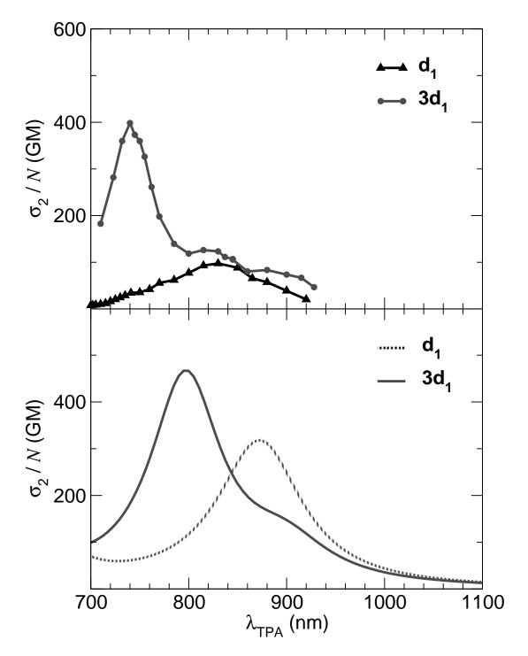
Figure 15: TPA cross section of chromophores  $d_1$  and  $3d_1$  normalized for the number of branches (N). Top panel: experimental data in toluene; Bottom panel: calculated cross section in vacuum, but corrected for local field and refractive index. Adapted from. [121]
