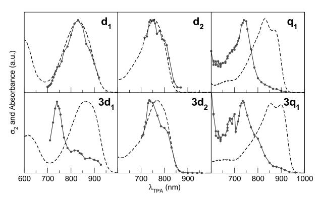
Figure 19: Experimental TPA (circles and lines) and rescaled OPA (dashed lines) spectra for monomeric compounds  $d_1$ ,  $d_2$  and  $q_1$ , and their corresponding branched systems  $3d_1$ ,  $3d_2$  and  $3q_1$  in toluene.
