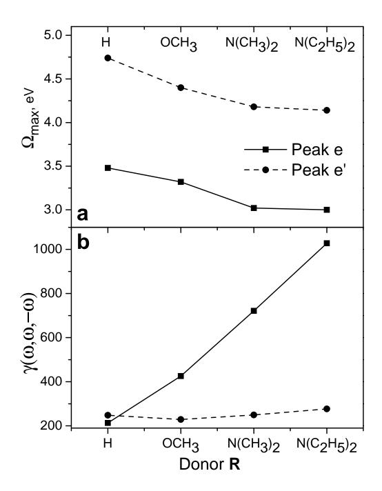
Figure 10: Variation of third-order polarizabilities (all  $\gamma$  are given in  $10^{-32}esu$ ) with the strength of the terminal donor groups for compounds  $q_4$ - $q_7$  in Fig. 7. The lines connecting the points serve as a visual guide. Adapted from.<sup>[194]</sup>
