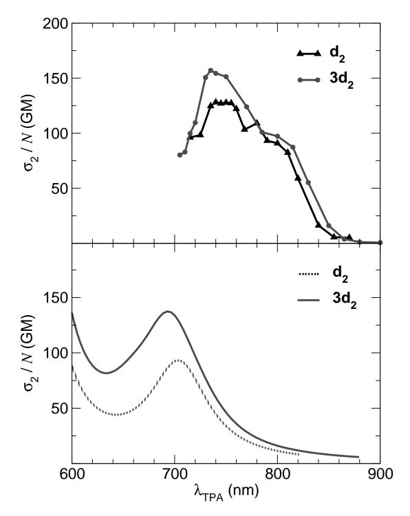
Figure 16: TPA cross section of chromophores  $d_2$  and  $3d_2$  normalized for the number of branches (N). Top panel: experimental data in toluene; Bottom panel: calculated cross section in vacuum, but corrected for local field and refractive index. Adapted from. [123]
