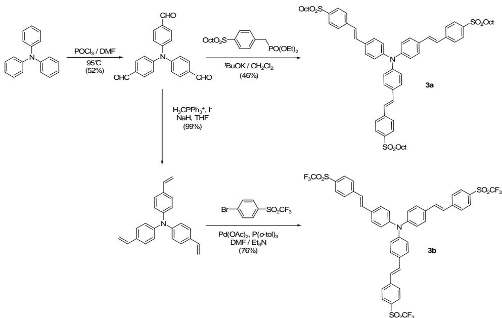
Scheme 2: Synthesis of octupolar chromophores **3a** and **3b**.
