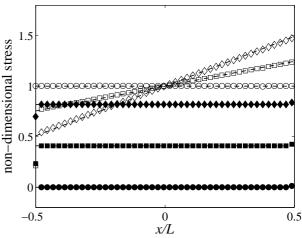
Fig. 2: Calculated stress fields  $\tilde{p}(\tilde{x})$  (open symbols), and  $\tilde{\sigma}(\tilde{x})$  (full symbols) for F=0 (circles), 0.41N (squares) and 0.82N (diamonds). Stresses are made non-dimensional by dividing them by the average pressure. For clarity, only 1 data point out of 9 is plotted. These fields are compared to the fields assumed in the model (dashed lines).
