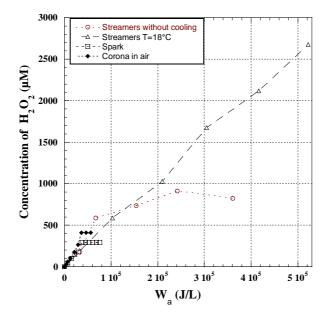
**FIGURE 4**. Production of  $H_2O_2$  versus accumulated input energy per litre  $W_a$ , for the 3 discharge types. Initial conductivity  $\sigma_0=100\mu$ S/cm.
