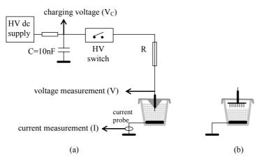
FIGURE1. (a) experimental set-up for streamer and sparks in water, (b) multipin test cell used for corona in air above the water surface. Current probe: 20 MHz current transformer (Rogowski coil).
