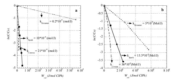
**FIGURE 5**. 4-chlorophenol removal versus accumulated energy per mole of pollutant ( $W_{rel}$ ) for the 3 pulsed discharge types. (a) without and (b) with 500  $\mu$ M of FeCl<sub>2</sub>
