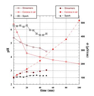
FIGURE 3. pH and conductivity variations versus time for the 3 discharge types in a pure water solution without organic pollutants, of initial conductivity  $\sigma_0=100\mu$ S/cm.
