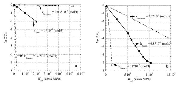
**FIGURE 6**. 4-nitrophenol removal versus accumulated energy per mole of pollutant ( $W_{rel}$ ) for the 3 pulsed discharge types. (a) without and (b) with 500  $\mu$ M of FeCl<sub>2</sub>
