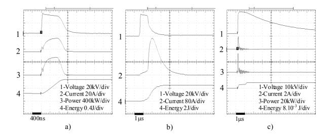
FIGURE 2. Typical electrical measurements obtained for streamer (a), streamer + spark (b), and corona in humid air (c)
