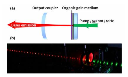
Figure 1 - a) Schematic representation of the plano-concave VECSOL resonator (see text for details). b) Long-exposure time photo of the working VECSOL.
