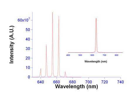
Figure 3– Typical emission spectrum of a 17- $\mu$ m thick active layer. Inset: single peak laser peration achieved for a 2.35- $\mu$ m layer.
