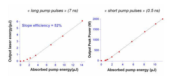
igure 2 – Output laser energy (left) and output peak power (right) vs. absorbed pump energy nder 7 ns and 0.5 ns pumping, respectively. The dashed line is a linear fit to the experimental lata.
