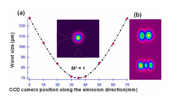
Figure 3 – a) Spatial evolution of the output beam profile along the emission direction. The dotted line is a fit to the experimental data with  $M^2$ =1. Inset:  $TEM_{00}$  laser beam profile. b)  $TEM_{10}$  and  $TEM_{20}$  images of the VECSOL emission obtained by fine misalignment of the VECSOL cavity.
