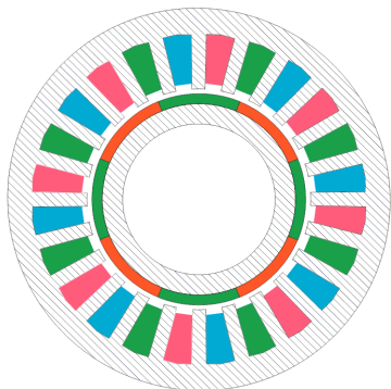
Fig. 1. Basic structure with 8 poles and 24 slots
