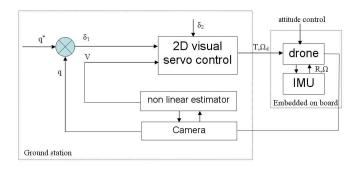
Fig. 5. Schematic block diagram of estimation and control loops.
