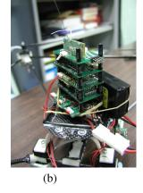
Fig. 3. The embedded camera (a) and the set of electronic boards (b).
