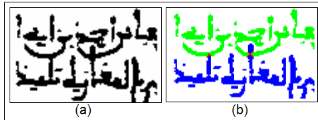
Figure 8. (b) Overlapping and touching connected components separation result of the window in (a).
