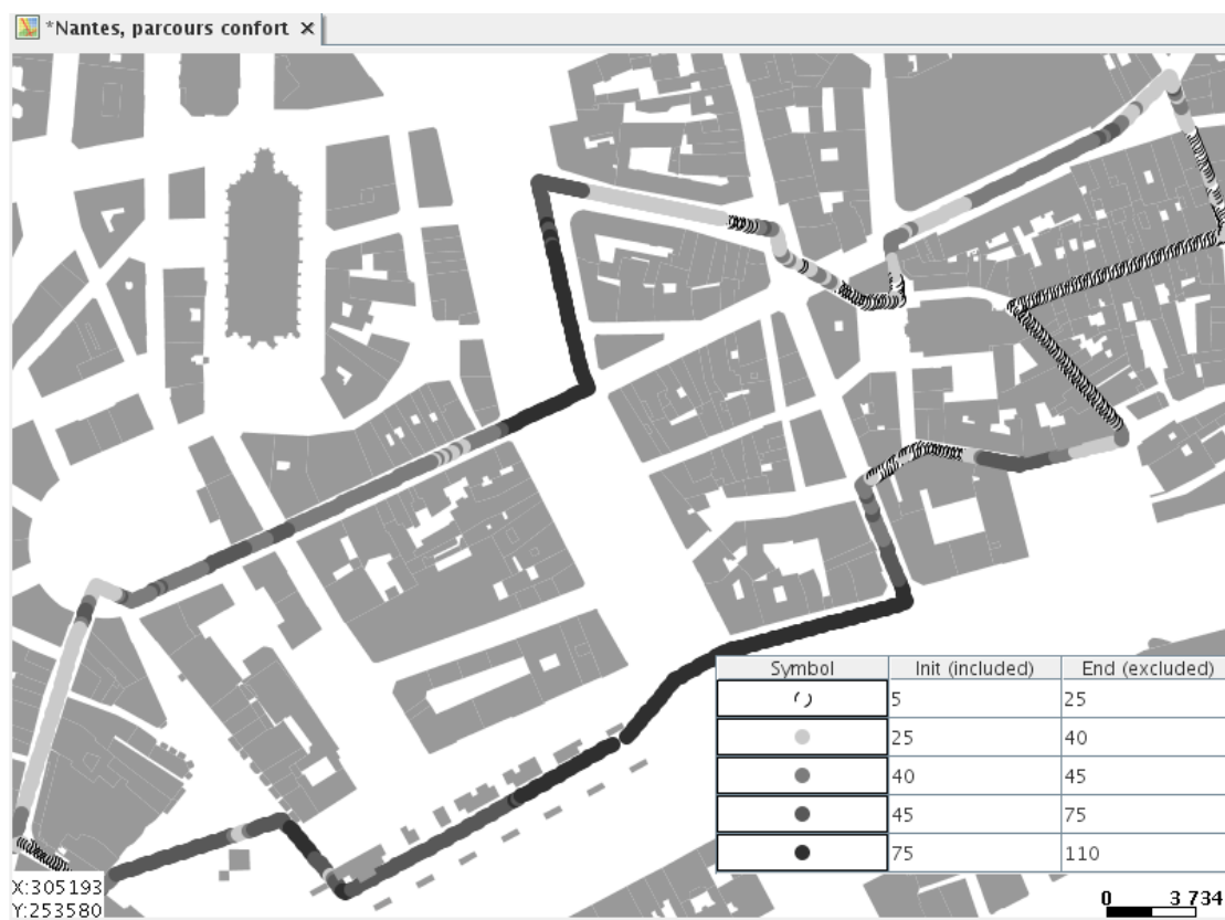
Figure 4: Interval classification of the isovist ray tracing approach with the 2nd order moment indicator. As may be seen in this figure, the values of this indicator in canyon streets (ranges 5-25 and 25-40) differ clearly from the values of the same indicator in open spaces like squares (ranges 45-75 and 75-110).
