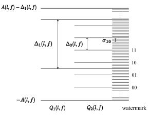
Fig. 4:  $Q_1$ - and  $Q_2$ -quantizers. A(l, f) is provided by the quantization of  $m_{max}^x(l, f)$  using  $Q_A(f)$ .
