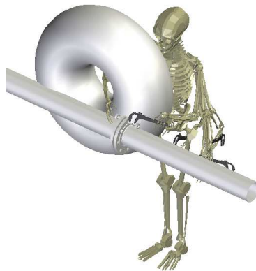
Fig. 9. Solution path for the first problem. The character only has to move its left hand.
