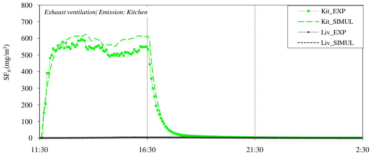
Figure 3. Exhaust ventilation - SF 6 concentrations for injection in the kitchen (Case A).
