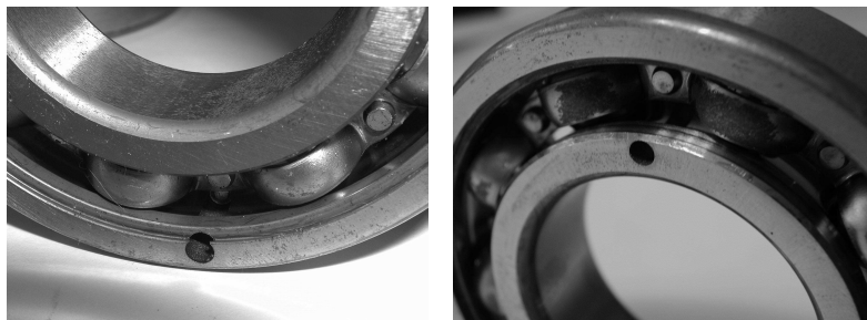
(a) outer raceway defect
