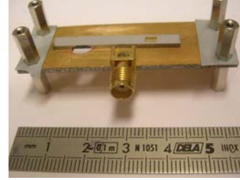
Figure 12. Test vehicle of a Si/LiNbO 3 PPT/Si device
