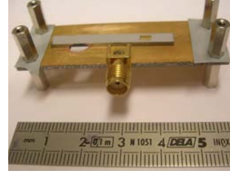
Figure 12. Test vehicle of a Si/LiNbO 3 PPT/Si device
