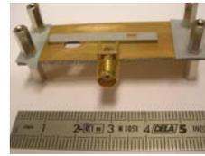
Figure 8. Test vehicle of a Si/LiNbO<sub>3</sub> PPT/Si device
