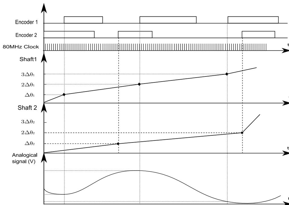
Fig. 4. Pulley angular rotations measurement principle.
