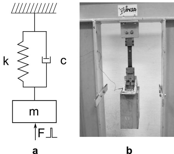
Fig. 10. Experimental set-up for the local belt characteristics identification.
