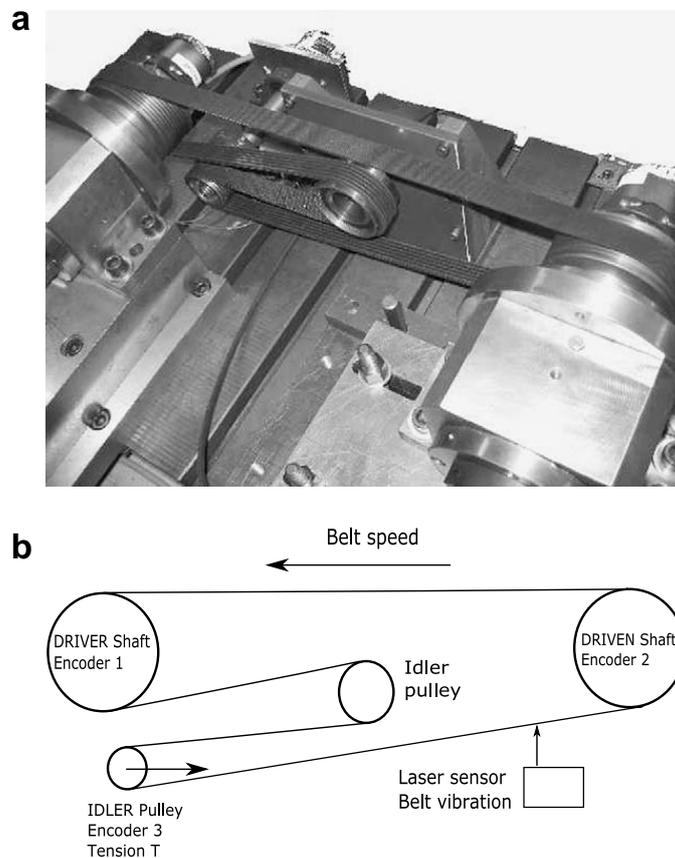
**Fig. 2.** Multi ribbed belt generic transmission set-up.
