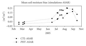
FIGURE 5: Comparison between surface soil moisture simulated and estimated from ASAR radar data. The domain average bias between the simulations and each ASAR image over Dantiandou Kori are shown
