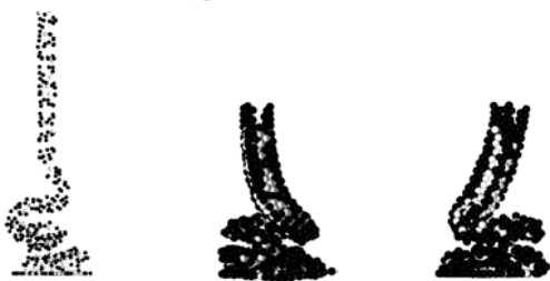
Figure 10: Particle type determination for paste simulation.
