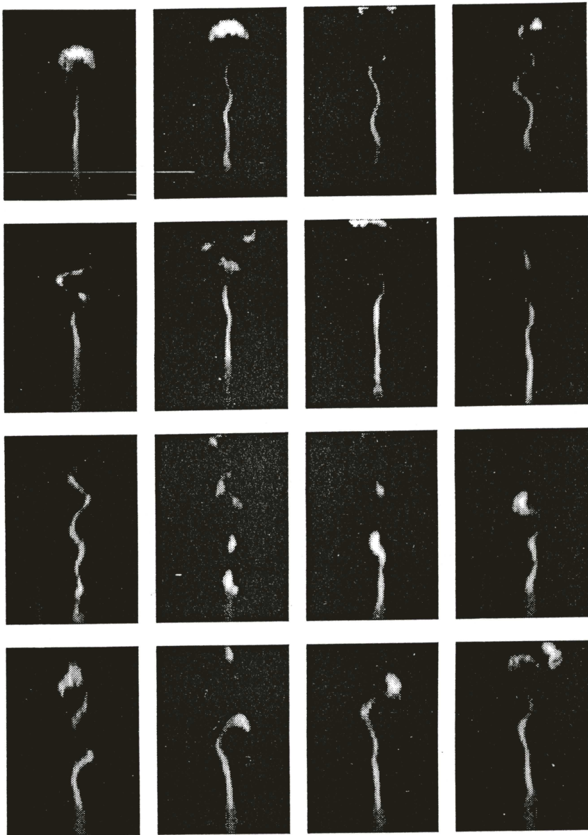
figure 16 A refined model of smoke. The time step of this chronogram is 1 sec
