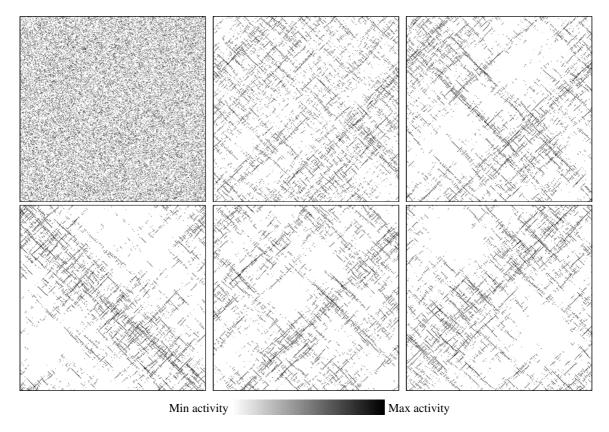
FIG. 7: Maps of cumulated plastic activity during "time" windows corresponding to increasing levels of deformation:  $\varepsilon = 0.01, 0.10, 0.20, 0.30, 0.50, 1.00$ . The system size is L = 256. While random at the beginning, the plastic activity progressively localizes along  $n_1$  and  $n_2$  directions.
