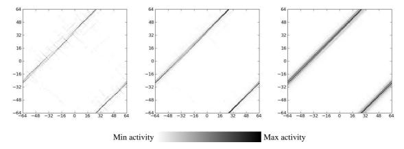
FIG. 13: Maps of total cumulated plastic activity corresponding to increasing levels of deformation:  $\varepsilon = 0.25, 1.0, 4.0$ . The initial threshold distribution is here shifted by  $\varsigma_0 = 0.5$ . The system size is L = 128. A clear persistent shear band can be observed.
