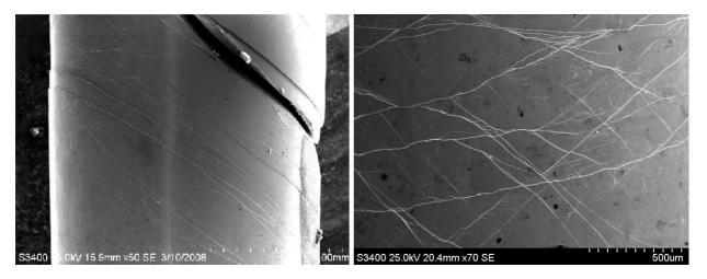
FIG. 1: Post-mortem Scanning Electronic Microscopy images of the side view of a cylindrical shaped bulk metallic glass specimen subjected to an axial compression. The left view shows a dense distribution of straight shear bands parallel to the final failure surface. The right one is a closer view of the cylinder side where the slip direction is mostly anti-plane. (Courtesy of J. Zhang and P. Aimedieu[12])
