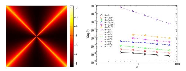
FIG. 11: (a) Power spectrum of the plastic strain using a decimal log scale. A clear quadrupolar symmetry is obtained. (b) Cuts along the axis at  $\theta = 0$  and  $\theta = \pi/4$ . Different power law behaviors  $S(q) \propto q^{-\alpha}$  are obtained between the extreme cases  $\alpha_0 \approx 0.33$  and  $\alpha_{\pi/4} \approx 1.67$ . L = 256 and d = 0.01.
