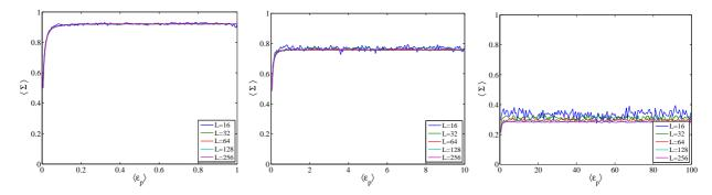
FIG. 3: Hardening curves: Averaged stress  $\langle \Sigma \rangle$  vs. plastic strain  $\varepsilon$  obtained for three values of the d parameter. (d=0.01 left, d=0.1 center and d=1 right). The curvature signs a clear hardening effect, i.e. the elastic limit (yield stress) increases with plastic strain. After the hardening stage, the stress saturates at a plateau value, the magnetic right strain.
