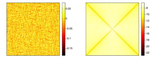
FIG. 9: (left) Stress map in the steady state, L = 256, d = 0.01. (right) Power spectrum (logarithmic color scale) of the stress map.
