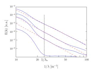
FIG. 4: (Color online) Spatial power spectrum E(k) of the velocity for  $P^{1/2} = 1, 5.2, 10.5, 24.7$  (from bottom to top). Dashed lines have slopes -4.6, -4.5 and -4.2 (from bottom to top). Dot-dashed line:  $\lambda_{\star}^{-1} = 25.2 \,\mathrm{m}^{-1}$  (see Fig. 5).
