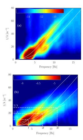
FIG. 1: (Color online) Space-time spectrum E(k, f) of the vertical velocity of surface waves: moderate (a) and strong (b) injected powers  $[P^{1/2} = 5.2 \text{ (a)} \text{ and } 24.7 \text{ (b)} \text{ in arb. units}]$ . Forcing: 1 - 4 Hz. Colors are log scaled. Solid white lines are  $\Omega_N(k)$  with N = 1, 2, and 3 (see text). Slope of the dotted line corresponds to a constant phase velocity  $\omega(k)/k$ .
