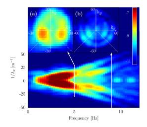
FIG. 3: (Color online) Space-time spectrum  $E(k_x, f)$  of velocity at  $P^{1/2} = 10.5$  located at  $k_y = 0$ . Same forcing bandwidth as in Fig. 1. Inset: space spectrum  $E(k_x, k_y)$  located at f = 5Hz (a) and 9 Hz (b). Dashed lines: forcing directions. Log scaled colors are different for each plot.
