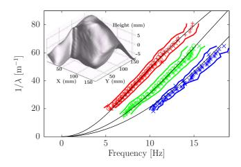
FIG. 2: (Color online) Nonlinear dispersion relation k(f) computed from the lines of maximum energy of E(k, f) for different forcings  $[P^{1/2} = 1 (+), 5.2, (\circ), 10.5 (\times), 24.7 (*)]$ . Solid thick lines around each branch correspond to the branch width averaged for all forcings. Solid lines are  $\Omega_N(k)$  with N = 1, 2, and 3 (see text - same as in Fig. 1). Inset: snapshot of the wave amplitudes at strong forcing  $(P^{1/2} = 24.7)$ .
