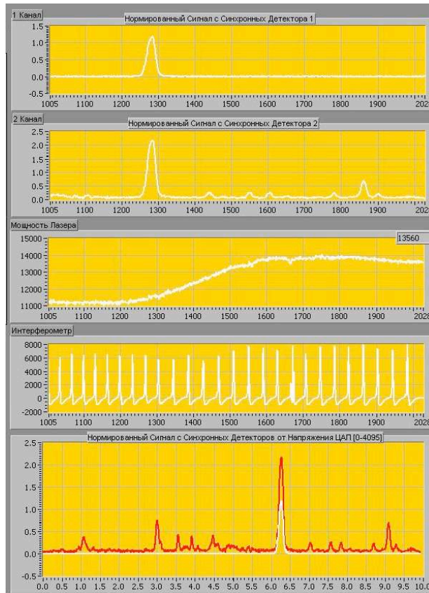
Figure 2: Menu of controlling and taking information from the two-channel spectrometer. See text for the description of the different traces.
