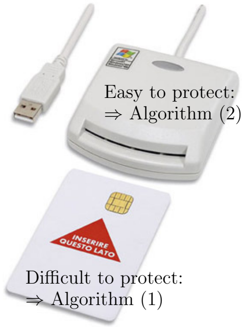
Figure 2. Probabilistic encryption is performed on the most vulnerable device while the deterministic decryption is safely carried out within the most secure device.
