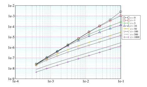
Figure 1: L<sup>2</sup> norm of  $\tilde{e}$  at t=1, as a function of the time step.
