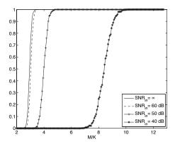
**Fig. 1.** Probability of reaching an output SNR greater than 30 dB as a function of the over-sampling ratio M/K. The results were obtained by drawing at random 1000 signals of length N=1024 and sparsity K=80. The number of measurements was varied from 2K to N-1.
