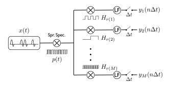
Fig. 4. Possible Analog Architecture.
