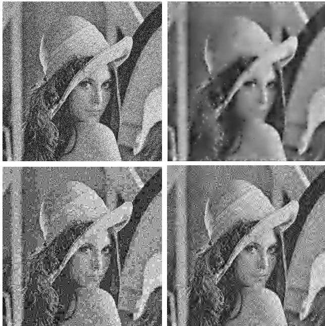
Fig. 4. Robustness to noise: qualitative comparison between our new codec, JPEG, and JPEG2000 under the same rate restriction (here 0.27 bpp). Upper left: Lena with additive Gaussian noise ( mean = 0 , variance = 0.05 for a normalized image dynamic range). Upper right: coded/decoded image using the new codec. Lower left: coded/decoded image using JPEG. Lower right: coded/decoded image using JPEG2000.
