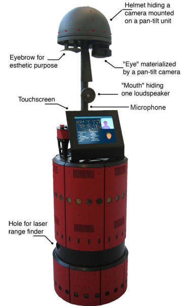
Fig. 4. Rackham and its equipment.
