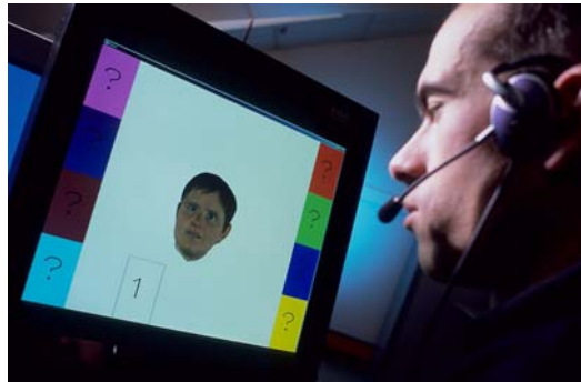
Figure 2 : Face-to-face interaction platform with an ECA (left) that provides deictic hints (see Figure 3) to a subject whose gaze is monitored. The hints help - or disturb - the subject in playing a virtual card game consisting of playing as fast as possible a card (white card here at the bottom of the screen) on one of eight possible positions (coloured boxes) according to different conditions.
