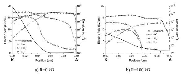
**FIGURE 2.** Influence of a resistor in series with a He-N<sub>2</sub> APGD: Electric field, electrons and ions distribution from the anode to the cathode when the current is maximum, for R=0 and R=100k  $\Omega$  (fluid model results)
