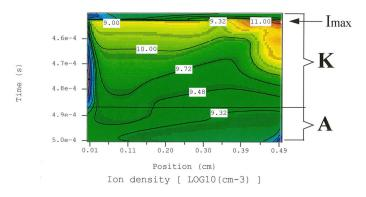
**FIGURE 5.** Space (anode to cathode) and time (one half cycle) distribution of the ions in a APGD in He calculated with a fluid numerical modelling [81]
