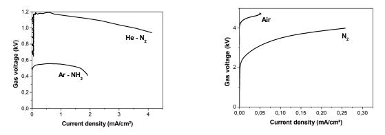
FIGURE 1. Gas voltage as a function of the current density during the current increase for He APGD ; Ar-NH<sub>3</sub> APGD ; N<sub>2</sub> APTD ; air APTD
