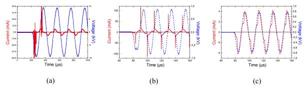
FIGURE 3. First discharges in (a)  $N_2$  APTD, (b) He- $N_2$  APGD (c) He- $N_2$  APGD with a current limitation. 10 cm<sup>2</sup> electrode area
