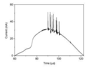
**FIGURE 6.** Microdischarges can develop after a Townsend breakdown. Current and gas voltage oscillogram of a N<sub>2</sub> DBD mixing an APTD following a Townsend breakdown and microdischarges developing after the current maximum when the  $\gamma$  coefficient is minimum and the current fixed by the power supply, the electrodes and the solid dielectrics.
